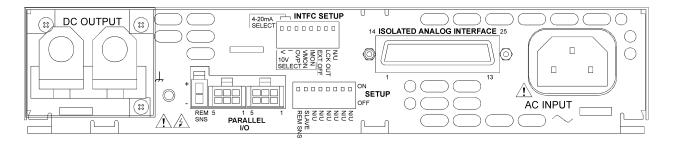
Figure 2–1. Rear Panel View, Low–Voltage Models
